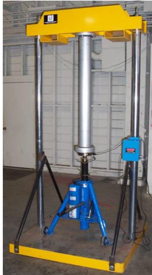
Our static Universal Jack Testers are designed to provide accurate load testing of both Tripod and Axle Jacks built by any hydraulic jack manufacturer. This tester is portable. An electronic load cell and digital electronic read-out provide easy and accurate readings. Rugged construction provides many years of continuous service, even in harsh environmental conditions.
