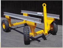
Rugged, simplified design permits higher net load capacities, at the same time insuring load protection under all transport conditions by virtue of the mixed springs rates involved in the combination of rails, frames and tires.
