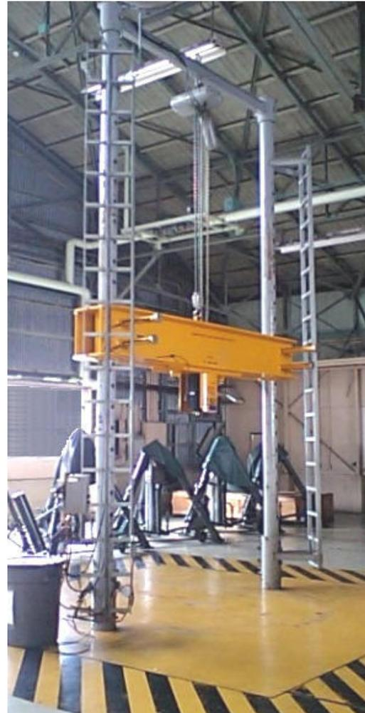
Our static Universal Jack Testers are designed to provide accurate load testing of both Tripod and Axle Jacks built by any hydraulic jack manufacturer. This tester is permanently mounted into the ground. An electronic load cell and digital electronic read-out provide easy and accurate readings. Rugged construction provides many years of continuous service, even in harsh environmental conditions.
